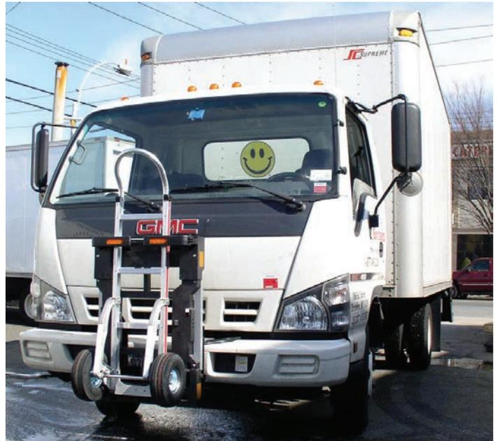
FIGURE 21: Front-mounted hand truck on truck.
