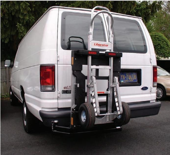
FIGURE 20: Rear-mounted hand truck on van.
