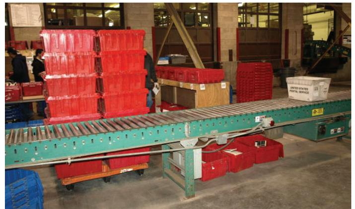
FIGURE 5: Gravity conveyor being used to unload totes.
