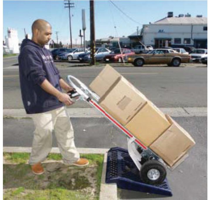
FIGURE 17: Hand trucks with brake and small portable ramp.
