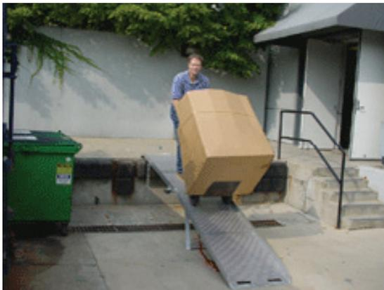
FIGURE 24: Portable ramps can be stowed under the truck or at the site.
