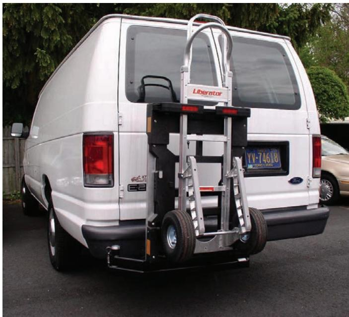
FIGURE 20: Rear-mounted hand truck on van.
