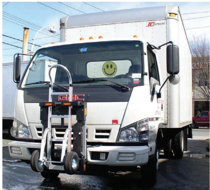
FIGURE 21: Front-mounted hand truck on truck.
