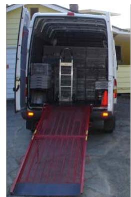
FIGURE 3: Tall vans equipped with portable ramps make tote handling more ergonomic and efficient.
