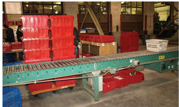
FIGURE 5: Gravity conveyor being used to unload totes.
