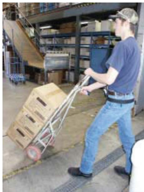
FIGURE 18: Hand truck with handle for better control.
