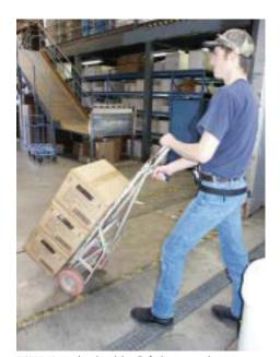
FIGURE 18: Hand truck with handle for better control.
