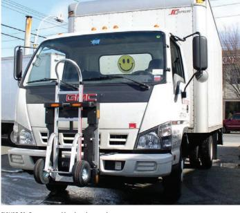
FIGURE 21: Front-mounted hand truck on truck.
