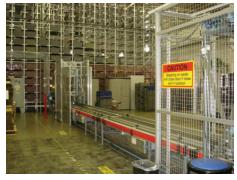
FIGURE 10: Totes are moved from large rack in background out to stacker/unstacker.
