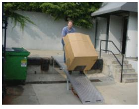
FIGURE 24: Portable ramps can be stowed under the truck or at the site.
