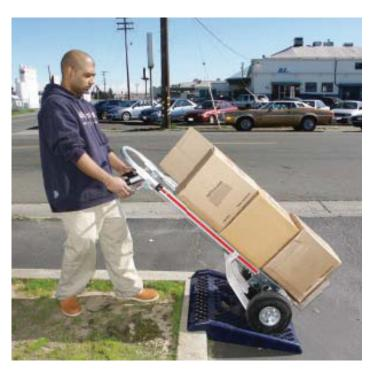
FIGURE 17: Hand trucks with brake and small portable ramp.
