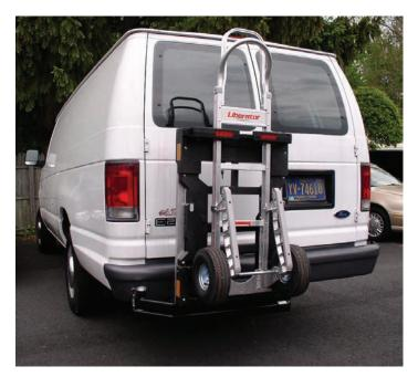
FIGURE 20: Rear-mounted hand truck on van.
