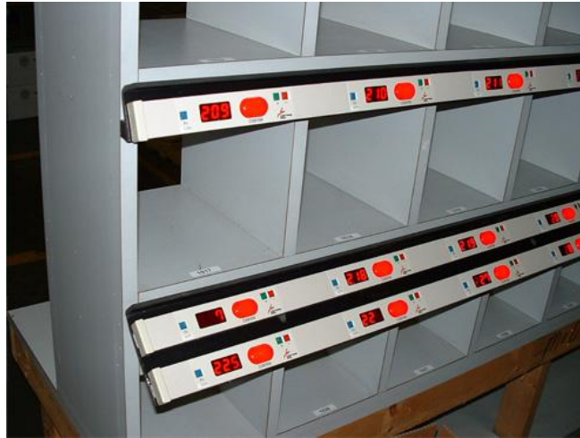
Photo 2: Pigeon-hole slots in put-to-light system
